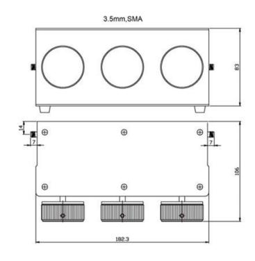
2WSA182106-8-99.9-\$ when frequency range DC~8GHz, 0~99.9dB attenuation range in 0.1dB steps, average power 2W, SMA connectors, are desired.
