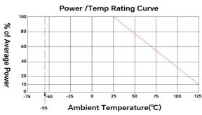
Datasheet Model Number : TMFA6410-XX *Coaxial Fixed Attenuator, DC-6.0GHz 1-40dB, 4.3-10 Male & 4.3-10 Female, 10W*
